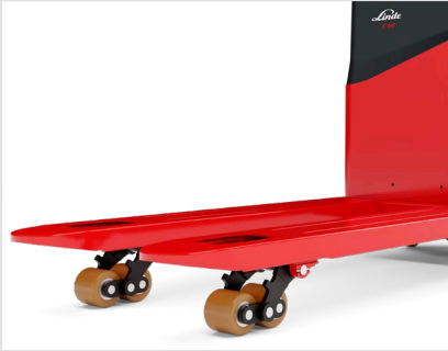
Castor wheels for additional stability
